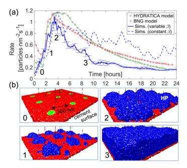
Hydration rate of cement paste: predictions from kinetic simulations at the nanoscale compared with results from existing models without submicrometre resolution
