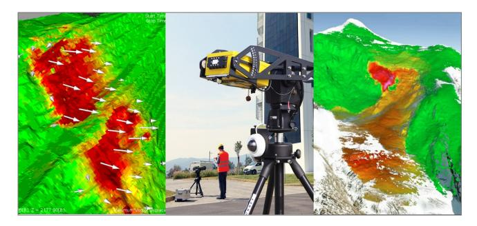
Ground-based radar interferometry (GBRI) is a remote sensing imaging technique based on coherent radar systems, which can measure not only the amplitude, but also the phase of the microwave signals. The phase measurements can then be exploited to derive information on the deformation and topography of the measured scene.
